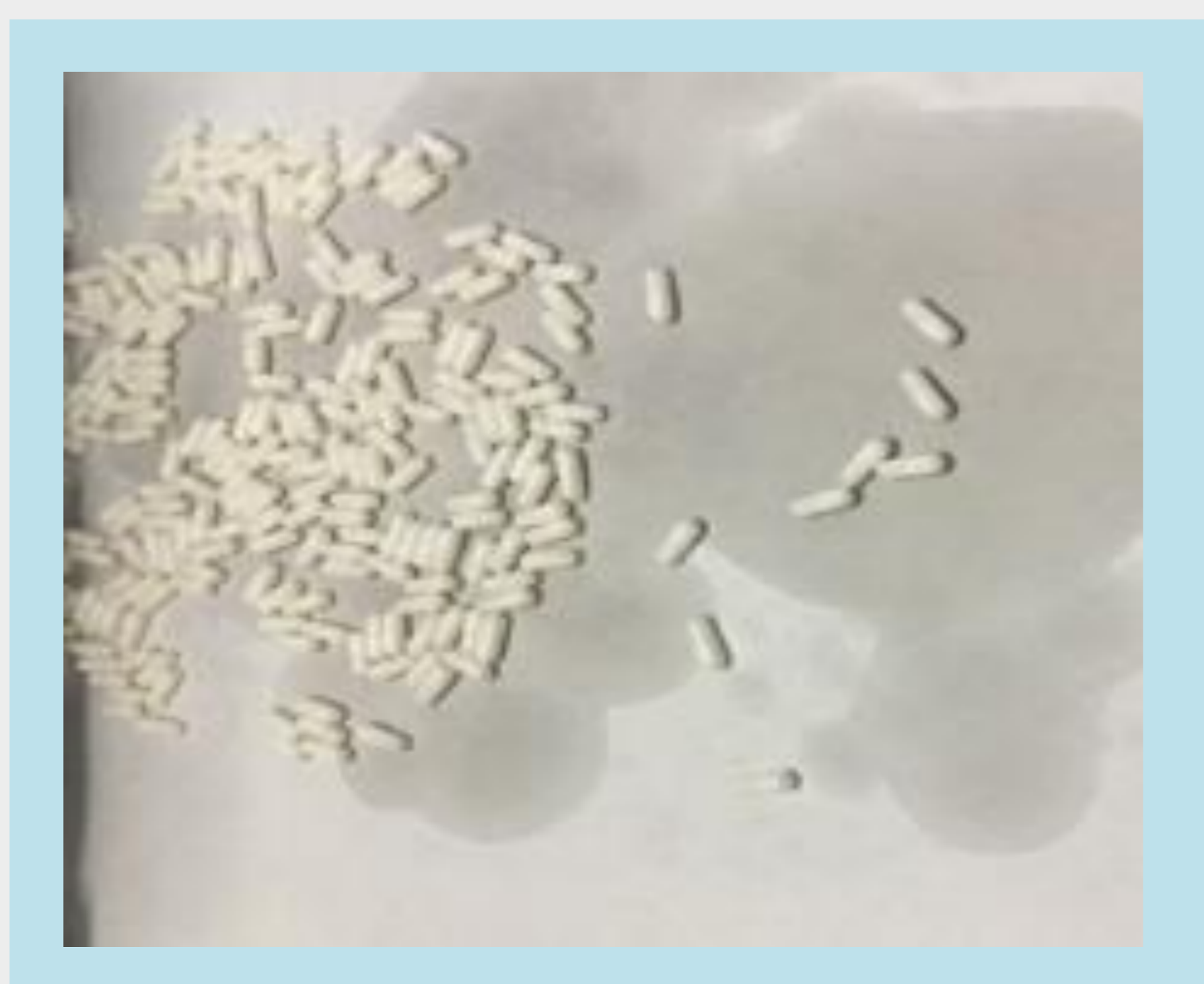
Figure 3 Extensive leaking for low viscosity product with a Conisnap® capsule
