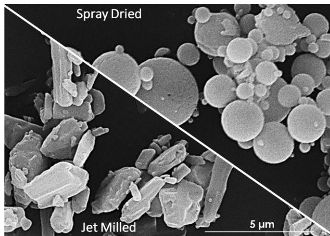
Figure 2 Particle morphology comparison for spray dried and jet milled mannitol
