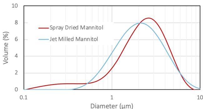
Figure 3 Comparison of time-of-flight aerodynamic particle size distribution for spray dried and jet milled mannitol
